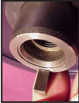
Re - Install harmonic balancer drive key.
