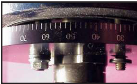
IMPORTANT ! Do not fully seat harmonic balancer against degreed drive plate before starting 3/8" washers and flange nuts.
