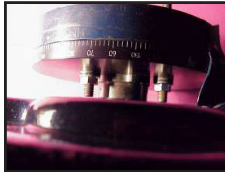
IMPORTANT ! Do not fully seat harmonic balancer against degreed drive plate before starting 3/8" washers and flange nuts.
