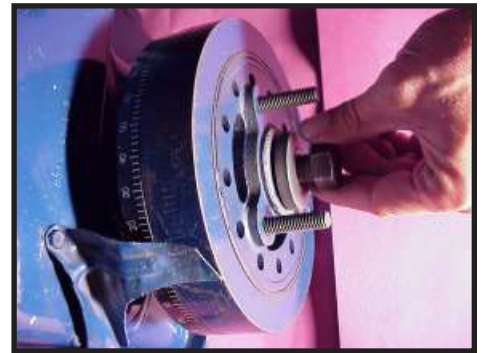
After 3/8" washers and flange nuts have been started, continue to install harmonic balancer using the center crankshaft bolt.
