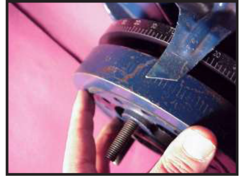
Install harmonic balancer. TDC should coincide with timing pointer.
