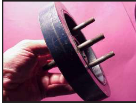
Install 3/8" drive studs into harmonic balancer.
