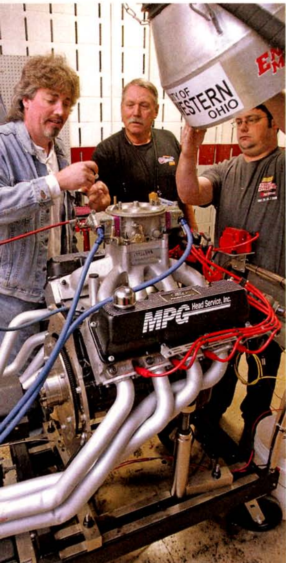
MPG Heads returned with the 400M that showed great potential, but wiped a camshaft in qualifying last year. This time the engine held together, and pulled the points for a fifth qualifying position going into the finals.
