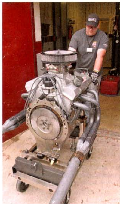
Among the many tasks handled by the students was uncrating the engines and mounting them to the test docking carts, and completing all dyno installations and hook-ups, then rotating engines on and off throughout the competition.
